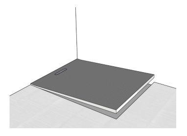
**4)** Position the shower element (1) in the screed recess, making sure the drain nozzle of the shower element (1) fits into the seal ring on the drain (4).
