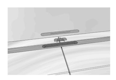
**15)** Fill the joint between the stainless steel drain channel (3) and the tiled surface with silicone.
