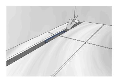
**12)** Once the correct height is set, insert the stainless steel drain channel (3) into the recess. Before doing so, carefully apply tile adhesive into the recess to ensure full-surface support for the stainless steel drain channel. Make sure no tile adhesive gets onto the blue sealing ring or into the floor drain.
