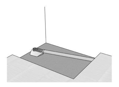
2) Fill the floor recess with levelling screed and level it flush with the top edge of the floor drain (4). The height difference to the screed equates to the thickness of the shower element (40 mm) + approx. 5 mm adhesive mortar. The resulting surface must be flat and horizontal.
