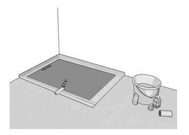
**5)** All connecting joints are sealed with the JACKOBOARD® 2-component sealing kit (or equivalent).
