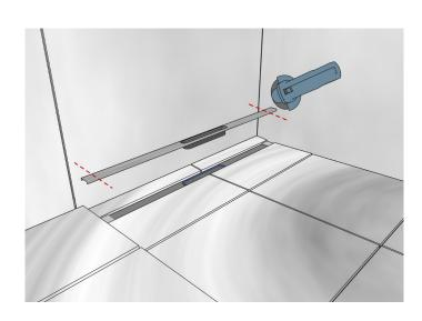
**9)** The stainless steel drain channel (3) should be flush with the tile surface. If necessary, the ribbed plastic base must be shortened. To do this, insert the stainless steel drain (3) into the blue sealing ring of the shower element (1) as far as it will go. Then measure the height difference to the tile surface.
