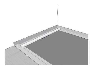
**6)** Before tiling the shower element, place the EPS tile block (2) onto the shower element (1) in the area where the drain channel is to be installed later. This serves as protection and as a drain place holder to facilitate tiling.
