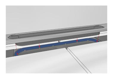
**14)** Place the hair trap (5) and the stainless steel cover into the stainless steel drain channel (3).
