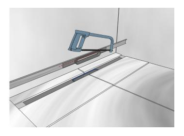
**10)** Shorten the plastic base using a hacksaw according to the measured height difference. Make sure that the cut is perfectly straight.
