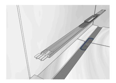
**11)** On the underside of the stainless steel drain (3), attach the supplied self-adhesive support blocks (6) at each end of the drain channel.
